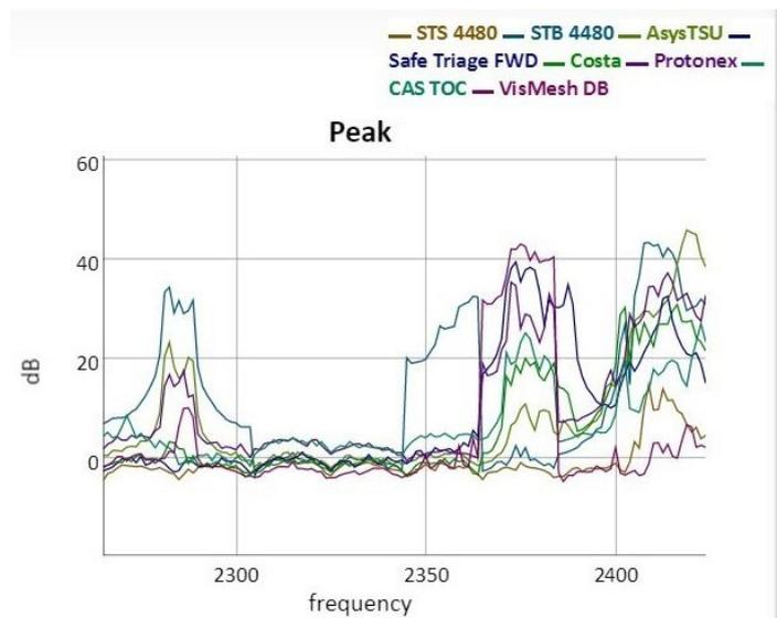
Figure 1. Network wide spectrum scan from the DSEI radios.
